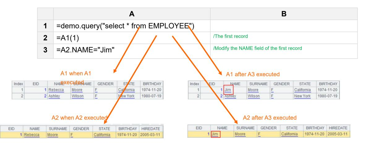
A2 is the pointer of the first record in set A1, and it is not the real data, when the data in A1 changes, A2 changes accordingly.
